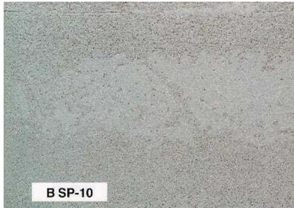
**Brush Off Blast SSPC-SP10 (SSI-Sa2 1/2), or NACE #2 Definition:**
